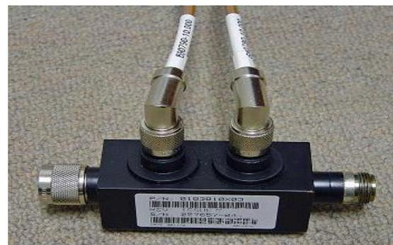
the characteristics of the directional coupler can be expressed in terms of its coupling factor and its directivity. Assuming that the wave is propagating from port 1 to port 2 in the primary line, the coupling factor and directivity are defined, respectively by,
